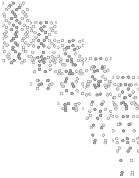
FIG. 8. Relative motion of random particle layer to fluid for initial thickness L_0/a=40 and \phi_0=0.060 .
